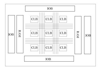
Figure 1: Typical FPGA architecture. The CLBs are the configurable logic blocks, IOBs are the Input Output Blocks and the RAMs are on-chip Random Access memory blocks.
